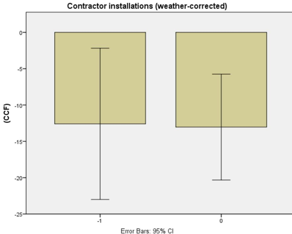
**Figure 20: Comparison of changes by method of installation (-1=contractor, 0=homeowner)**
